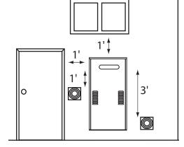
Figure 1: Discharge Vent Clearances.
